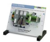
AXC F 2152 starter kit including PLCnext Control AXC F 2152, voltage switch, digital input and output module, analog input and output module, potentiometer, switch module, PROFICLOUD license, as well as a power supply unit, patch cable, country-specific adapter plugs, and documentation.
